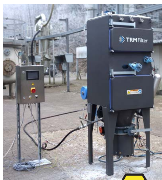
ECR unit during explosion tests at the FSA site in Germany
