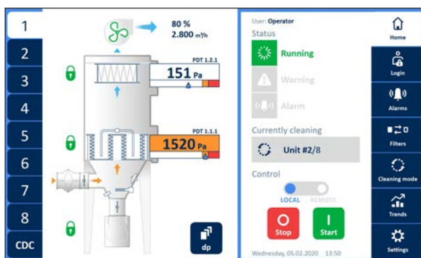
Graphical user interface of the standard ROTATRONIC Control (the user interface of the ROTATRONIC Control LT offers an alphanumeric display)
