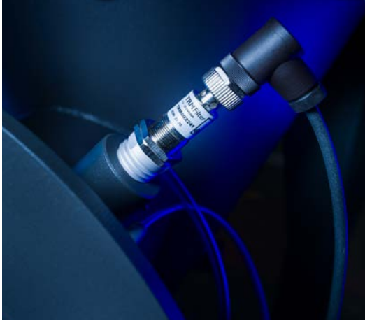
Explosion detection sensor on ECR dust collector
